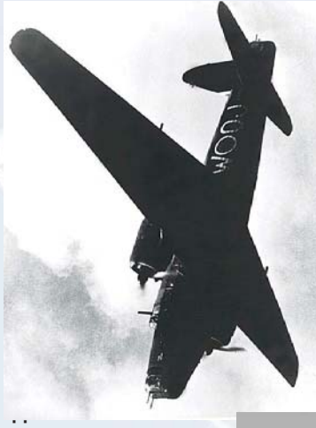
Vickers Wellington P = 2 x 1055CV Vmax = 410km/h Plafond = 6700m Charge utile = 2040kg
