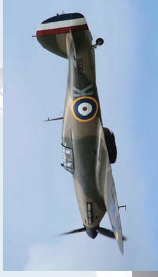
Hawker Hurricane P = 1300CV Vmax = 510km/h Plafond = 11000m Charge utile = 800kg
