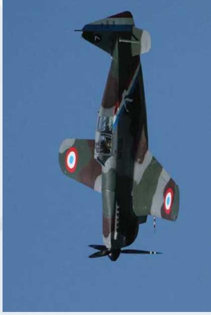
Morane Saulnier MS406 P = 860CV Vmax = 486km/h Plafond = 9850m Charge utile = 700kg
